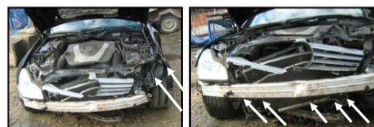
Figure 3. Display of the damage of the upper left-hand cooler "connecting bracket" [3]
