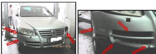
Figure 23. and Figure 24. Damage to the front bumper and "tear" of the front bumper [3]
