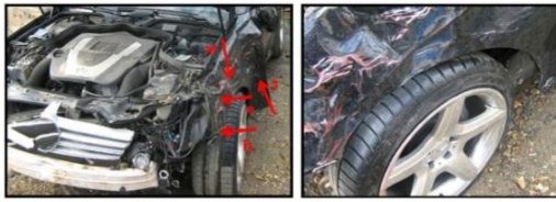
Figure 5. detailed damage left fender [3]
