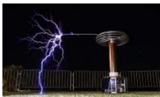
Figure 4. Electric shock of the Tesla transformer, source
