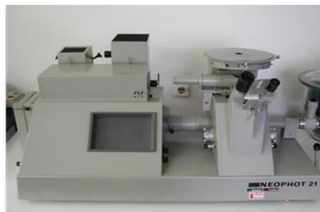
Figure 1. Metallographic microscope "Carl Zeiss" type "Neophot 21" N°22984 - "ORAO" AD. Bijeljina
