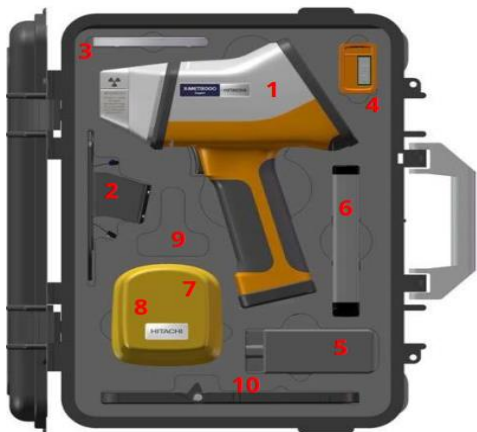
Figure 6. Appearance of portable handheld analyzer X-MET 8000 Alloy Expert "HITACHI"; № 804280 "ORAO" A.D. Bijeljina
