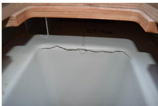
Figure 1. Damage to the keel (Source: Authors 2018)
