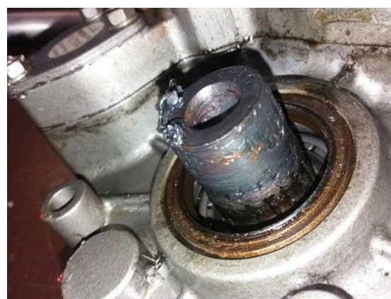
Figure 3. Damage to the engine clamp (Source: Authors 2018)
