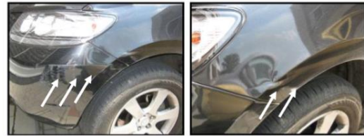
Figure 17 and Figure 18. Display of front bumper damage and scratch marks [3]
