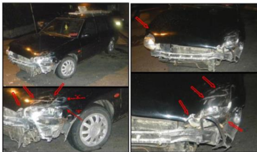
Figure 29. and Figure 30. Widely looks at the damage to the front left mudguard and shows a closer look at the damage to the front left mudguard [3]
