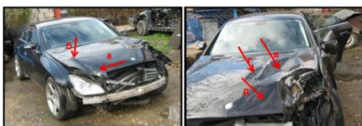
Figure 1. Width appearance of engine bonnet damage [3]
