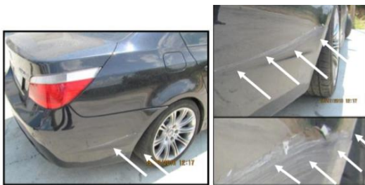
Figure 13. and Figure 14. Scratches on the rear bumper and cracks on the right-hand side of the rear bumper [3]
