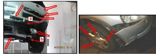
Figure 25. and Figure 26. Characteristic damage of decorative plastic and Damage to the front left wheel wheel [3]
