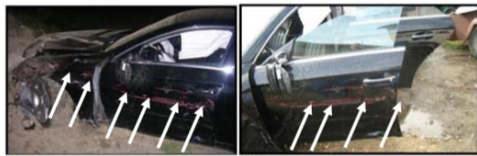
Figure 7 and Figure 8. Damage to the front left mudguard and front left door [3]
