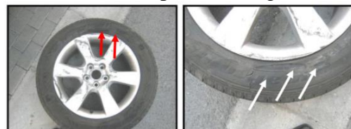
Figure 21 and Figure 22. Tire damage display [3]
