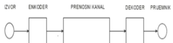
Figure 1. General information system view
