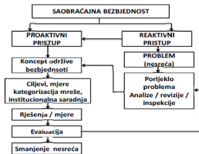
Figure 3. Proactive and reactive approach to improving road safety through road design
