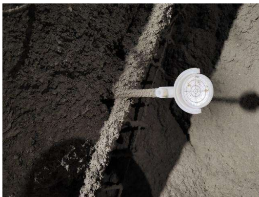
Figure 4. Prism reference point/crown (photo by N. Halilbegović, 2024.)
